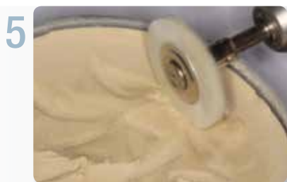
Using a soft 15 mm bristle brush, spin brush in polishing agent to incorporate paste into brush.
