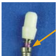
fig. 2b In dynamic fatigue testing, the titanium implant failed before the cemented interface between the Lava™ Zirconia and titanium, demonstrating the bond strength between Lava zirconia, RelyX™ Unicem Cement and the titanium abutment. 3M ESPE, 2008.
