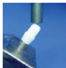
fig. 1a Applying force at a 30° angle. 3M ESPE, 2008.
